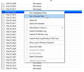
The tool will prompt the user as to which card they need to use for this test. For example, by running the Test VISA.TC.0013 above the tool requires the VISA CONTACT TEST CARD
