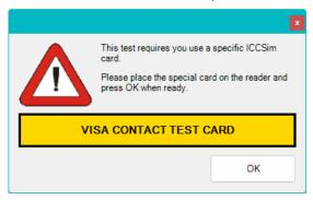
The user needs to place the specific card on top of the reader. Once the card is on top of the reader you can click on **OK** and the script should load to the card – this process takes around 1-2 seconds.
