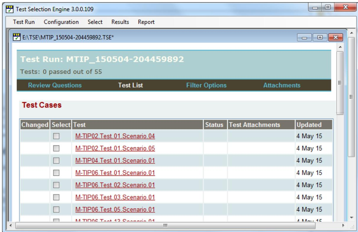
The MasterCard TSE tool can create the test list as either a **.tse** file or a **.tsez** file. The **.tsez** file is required for import into TMat. Please ask your acquirer to send the test list in the **.tsez** format.
